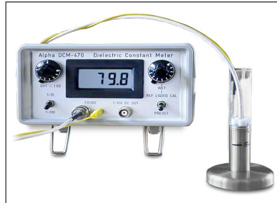
These pictures show how easy it is to measure the absolute Permittivity (Dielectric Constant) of liquids with our new DCM 470. Here, 5ml of water is examined in a 16mm glass tube.
